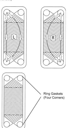
The following are some typical flow arrangements found in plate heat exchangers:
