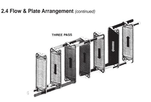
The connection locations may vary for a given plate heat exchanger design. Since all of API Schmidt-Bretten plate heat exchangers are parallel or same side flow, all connections for one fluid will only be on the right side and for the opposing fluid on the left side. The connection locations are defined as follows:
