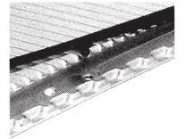
The circular ring portion of the gasket prevents the fluid from going across the thermal plate and sends it on to the next open plate or channel. The remaining field portion of the gasket channels the opposing fluid across the plate / heat transfer surface.
