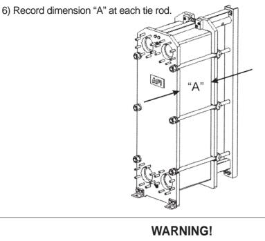
The tightening dimension "A" is critical for proper sealing of the heat exchanger. Be certain to record it accurately!!
