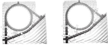
Any fluids escaping from either side will exit the heat exchanger through these vents. These openings must not be plugged as cross contamination of fluids could occur.
