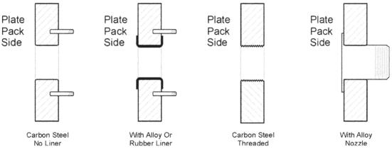
Threaded studs secure the flanges to the fixed frame plate. Alloy or rubber linings are added as necessary to prevent corrosion.
