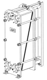
5) The plates can either be sequentially marked as they are removed from the unit or a diagonal line can be drawn across plate pack to record each plate's position.
