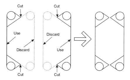
Certain plate models (S26, S27, S66, S76, S96, S106, S108, S114, S136, S138, S149, S156, S229, SX29, SX49) require a special endplate gasket, as shown.
