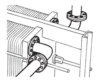
• The pressure plate must move backward for servicing. Use elbowed spool pieces for easy removal.
