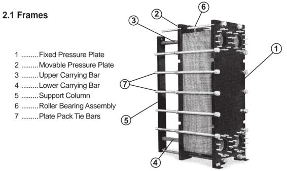
The fixed frame plate (1) and the moveable pressure plate (2) are dense steel plates designed for withstanding high pressures and containing the fluid connections.
