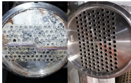
TUBE SHEET BEFORE & AFTER
