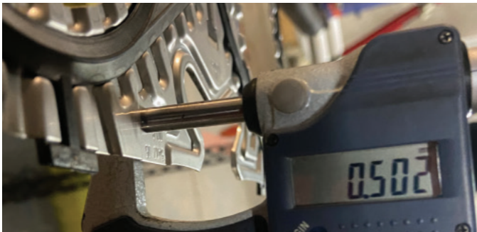
DIRTY PLATES / CLEANING OFF DYE ACID WASHED PLATES / VERIFYING PLATE THICKNESS
