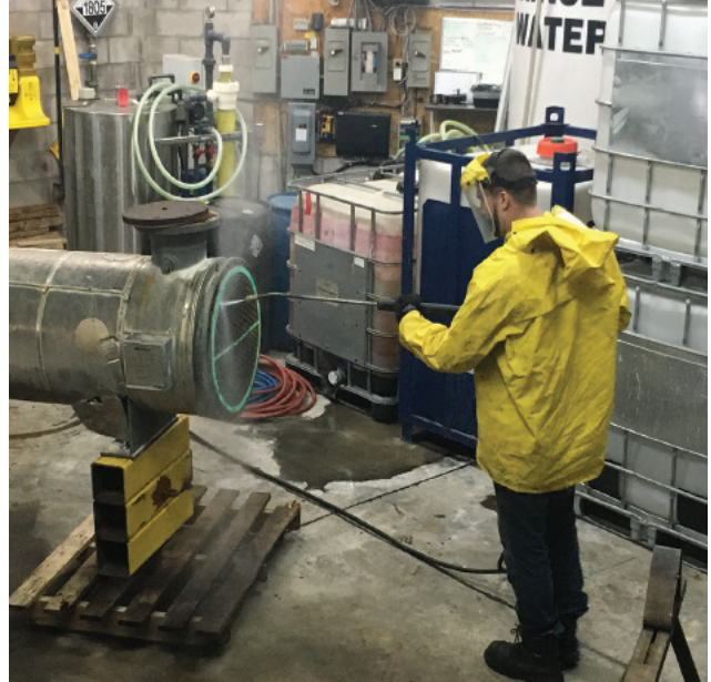
PRESSURE WASHING, CHEMICAL CLEANING
